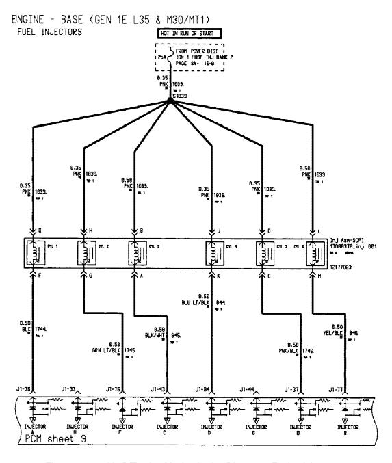
Figure 3.2.1a - V - P/Truck - Mechanization Diagram - Engine Injectors
